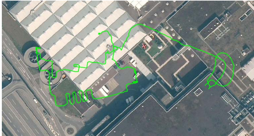
Environment with magnetic field disturbances: track is completely distorted
