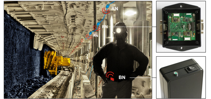
Fig. 3. Infrastructure components for RSS-based positioning and tracking of maintenance staff in the underground longwall coal mining environment (RN – reference node, BN – blind node).
