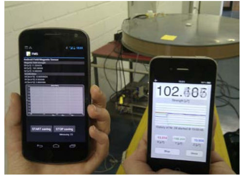
Figure 8: Customized Applications for MILPS measurements running on Samsung Galaxy (left) and iPhone 4 (right)
