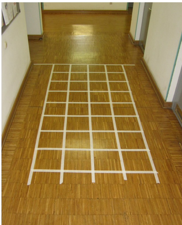
Fig. 6: An evaluation of the position estimation error of the RS in a corridor of our building. 5 \times 9 grid positions are marked in 30 cm intervals.
