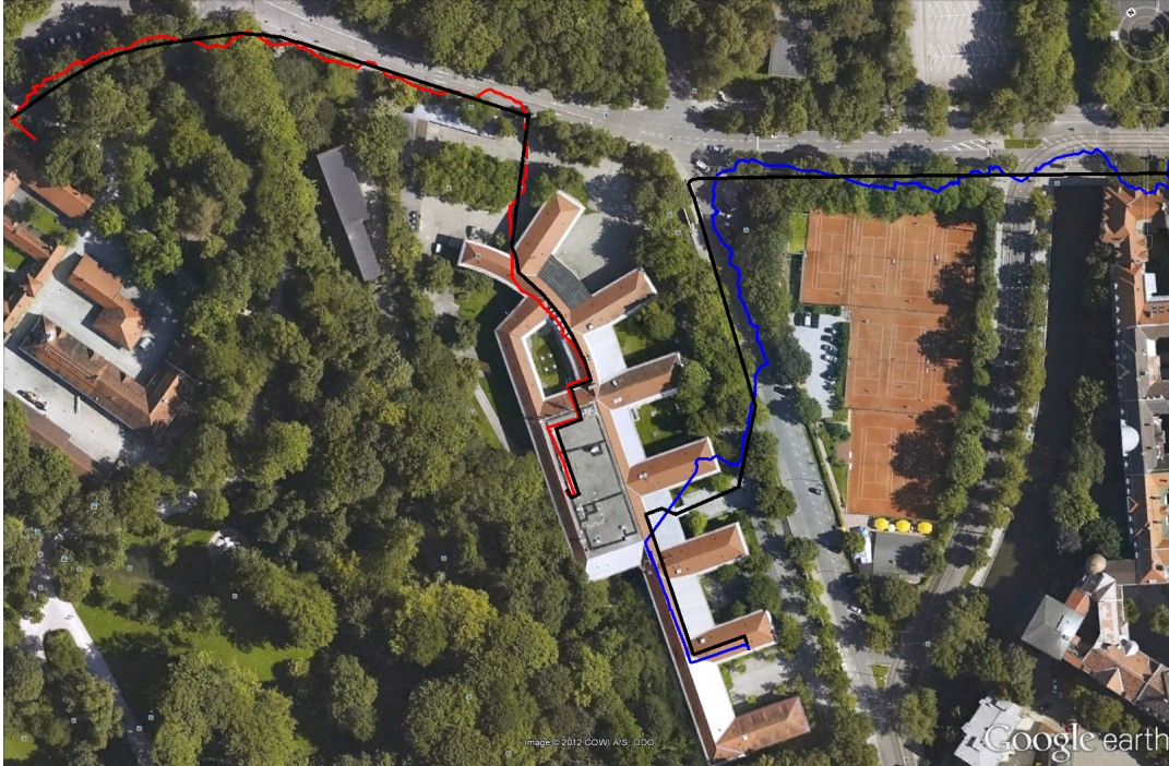
Figure 3: Two tracks corresponding the scenario, estimated track in red (left) and blue (right), real tracks in black.
