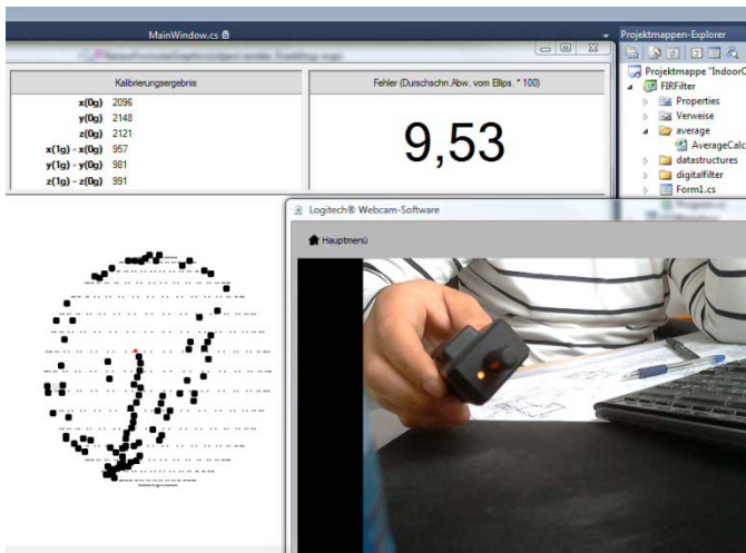
Figure 5. Software for the determination of the measured values, Visualisation of the radius and of the resulting calibration value during a free motion around the wrist using the Bodyguard-System.
