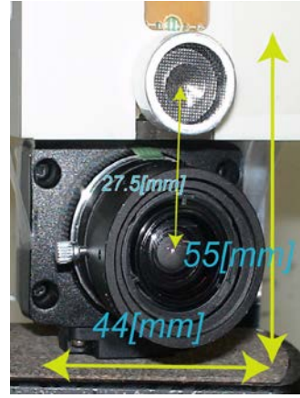
Figure 8: A receiver unit including a camera and an ultrasound receiver. Their baseline is 27.5 mm.
