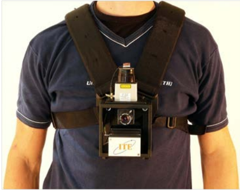
Fig. 1: Multi sensor pedestrian navigation system with IMU, Barometer, and Magnetometer with additional sensors (laser ranger, camera).
