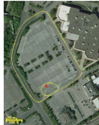
Figure 5. Transmitter (red square) and trajectory of the mobile receiver (original photo from Google Maps)
