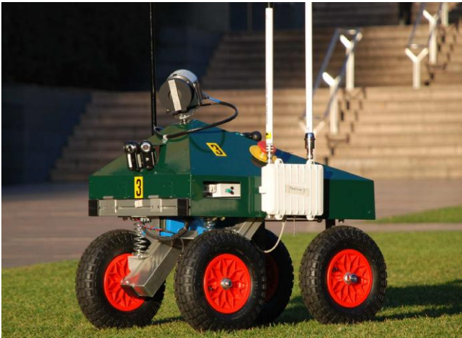
Figure 1. A picture of The platform. A LMS2151 laser scanner can be seen at the top of the platform.
