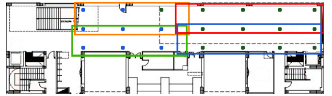
Fig. 4. Experimental environment. Colored dots indicate the RSSI clusters. Colored rectangles identify the 3D sub-models defined including orientations.
