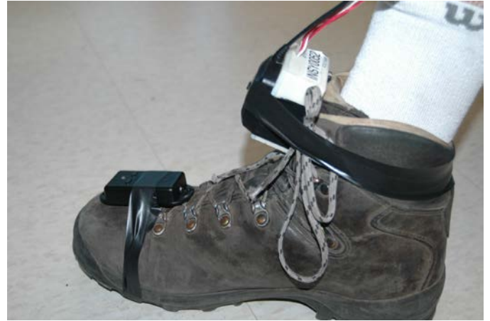
Figure 12. Subject's Foot with Two IMU's and Antenna
