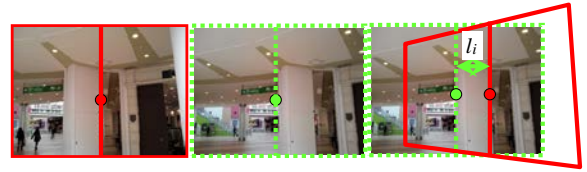
Figure 2. Viewing direction estimation. The left shows the query image. The center shows the reference image in the database. The right shows the projection of the query image to the reference image using the homography parameters (red rectangle).
