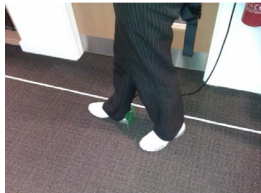
Figure 2. Mapping RFID Tags Using Foot-Mounted Antenna and Tape
