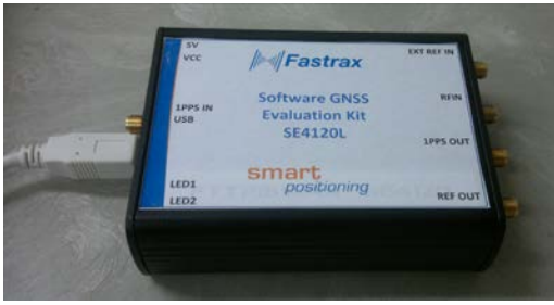
Figure 4. Radio front-end of the Fastrax software GNSS receiver used for pseudolite signal tracking
