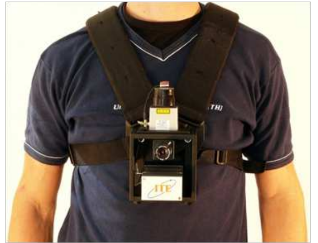
Fig. 4. Torso system with IMU, baro, magnetometer, laser ranger and camera
