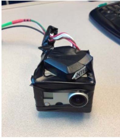
Figure 9. Data set 2 set up with the IMU, GPS antenna and camera attached. The system was located on the user's ankle.
