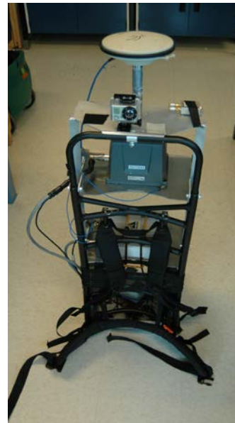
Figure 6. Data set 1 set up with the IMU and the camera located on the backpack.
