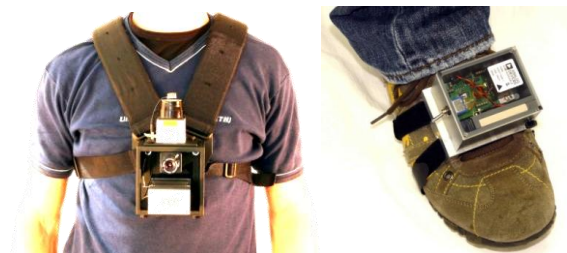
Fig. 1: Dual IMU system: with GPS, laser, camera, IMU, MAG, BARO and a foot IMU
