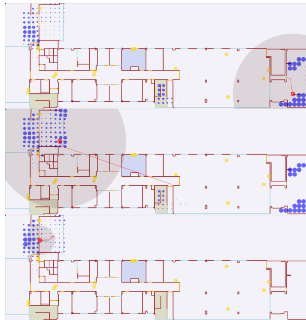
Fig. 5. First of a series of five consecutive snapshots walking along the path depicting the value of the likelihood observation function (blue circles) and the estimated position (red circle) for all three algorithms, i.e. using only the Gaussian (top), using the Gaussian and estimating the attenuation explicitly (middle), and using the Gaussian with attenuation estimation as well as modeling the pickup probabilities as Gibbs distribution (bottom). The top two likelihood functions show a strong multi-modality making the position estimation ambiguous. Because different devices were used for fingerprinting and for localisation the intermediate likelihood function yields a bit better likelihoods in the true position on the top left corner, however only the introduction of the Gibbs distribution explicitly modeling the pickup probabilities removes the dominant second mode from the density function resulting from the lower number of covering access points on the right hand side of the building.
