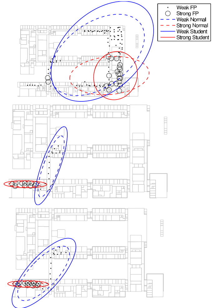
Figure 2: Three examples of two-level coverage area models fitted using normal and Student-t regression. In the first example the two strong FPs in left hand side affect strongly on normal model while the Student-t is not affected that much. The second and third examples show the difference of CAs if the strong FPs are included or excluded from the weak CA.
