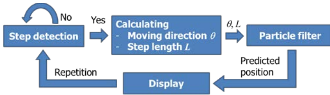
Figure 6. A block diagram of the developed navigation App
